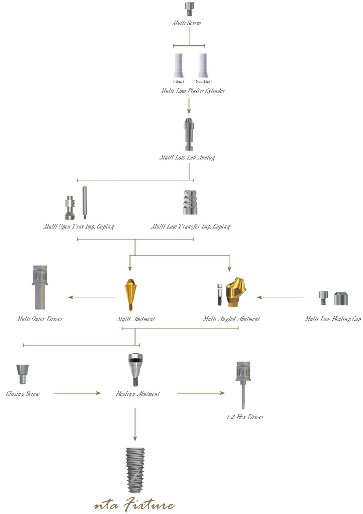
NTA PROSTHETIC FLOW DIAGRAMS FOR NTA SYSTEM
